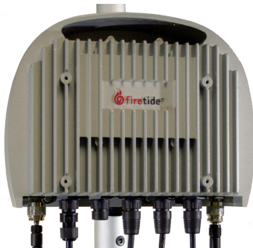
Figure 2. HotPort Outdoor Node Mounted on Pole
