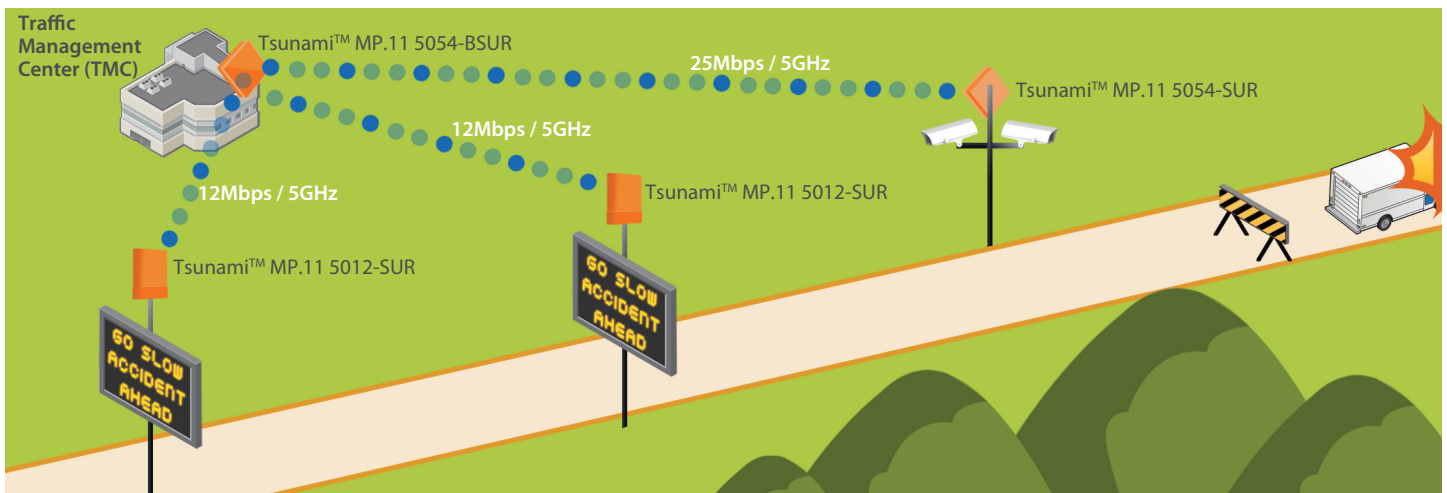
Figure 1: Variable message sign boards powered by Proxim wireless backhaul products
